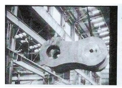
At left is a web assembly complete with journal pin. The smaller hole to the right in the pin is for oil lubrication of the white metal connecting bearing. This assembly is being moved up shop to the horizontal borer for final machining of the bores on the left.
