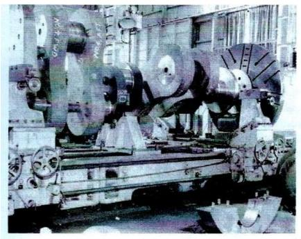
This photo shows a two-cylinder section. The crank journals can clearly be seen, one on the left in the vertical position and the other central at almost 90 degrees. This is the aft section of the crankshaft as the right tool-box is set at the trust block flange which takes the trust of the propeller. Without this flange the propeller would virtually drive the shaft clean out though the front of the engine.
