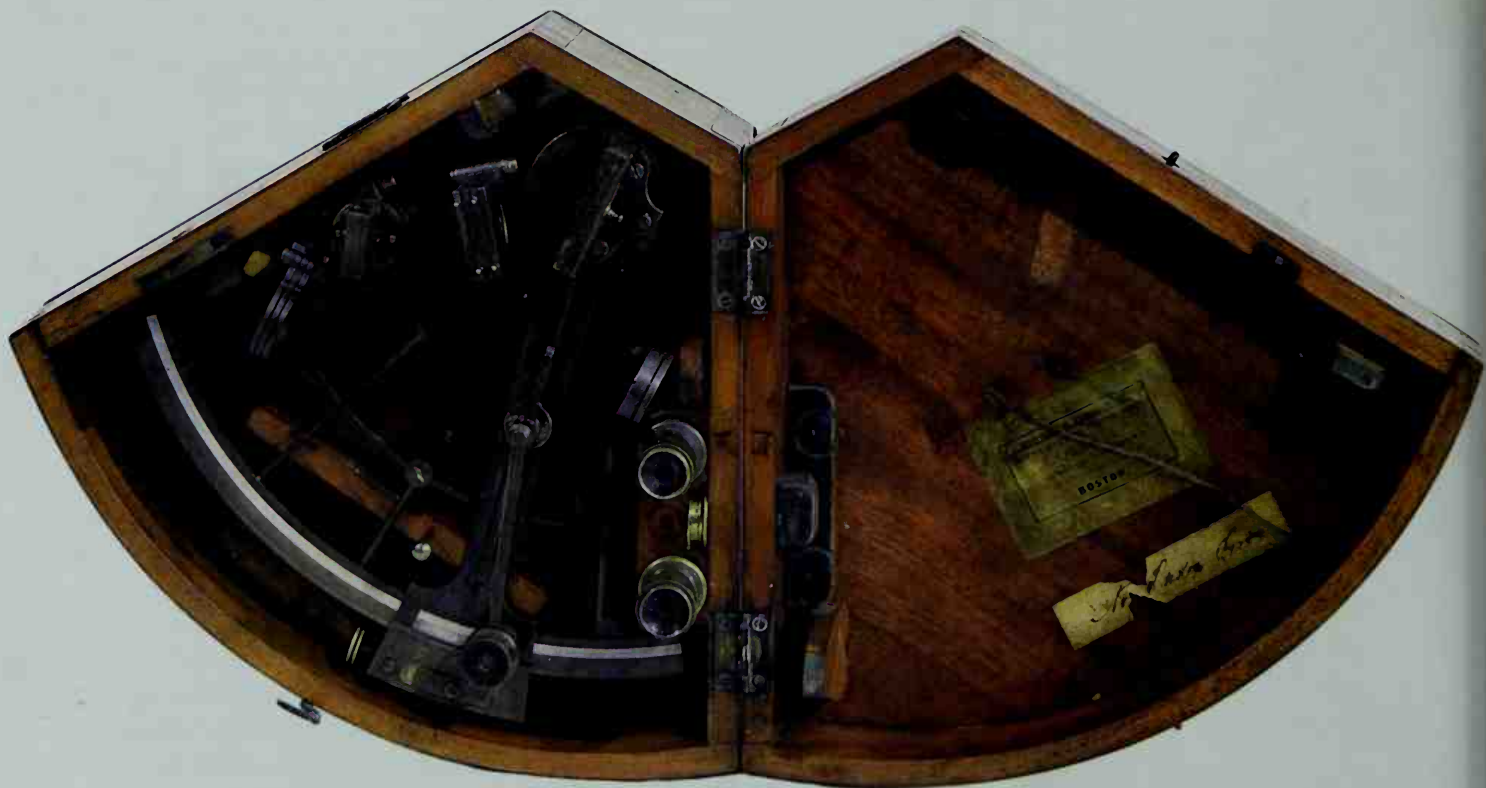
The sextant measured the angle of celestial bodies above the horizon. After making sextant sightings and noting the time, the captain used his nautical almanac to calculate his position.
