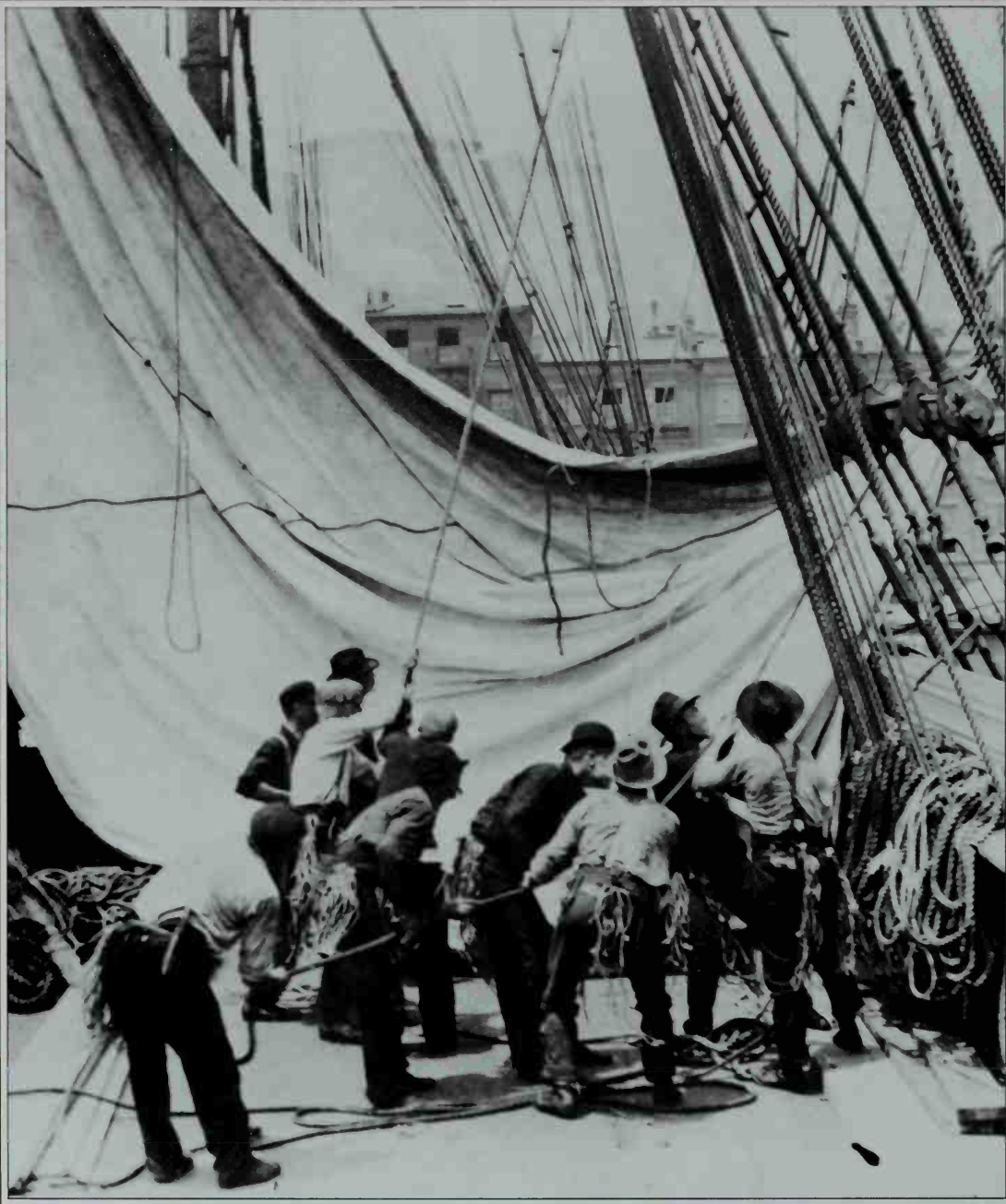
Readyng the Roanoke for departure, a shore gang of professional ship riggers starts hoisting a square sail by hand (above), then uses the ship's large capstan (right) to winch the heavy canvas up to its yard. Altogether, the Roanoke carried 15,000 square yards of canvas on four masts, including a 95-foot-wide mainsail that weighed half a ton when dry—and about twice as much when wet.
