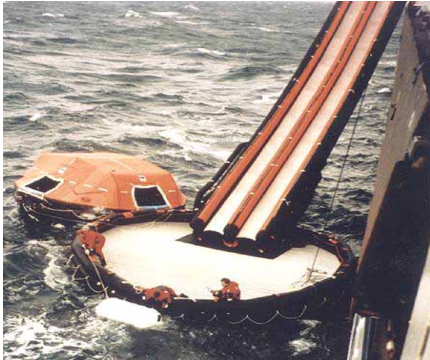
Marine Evacuation System, dual-track slide platform, 50 person liferaft.
