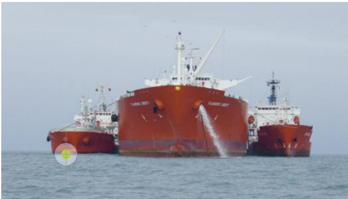
Ship-to-ship transfer from the FLANDERS LIBERTY , LPG carrier, 84,500 cbm, delivered in 2007 by South Korean shipyard Daewoo, operated by Belgian shipowner Exmar
