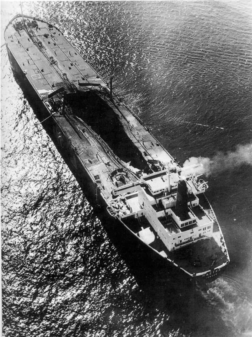
Figure 2.4: Mactra deck after tank cleaning explosion. Two killed. Source: Auke Visser, supertankers.topcities.com
