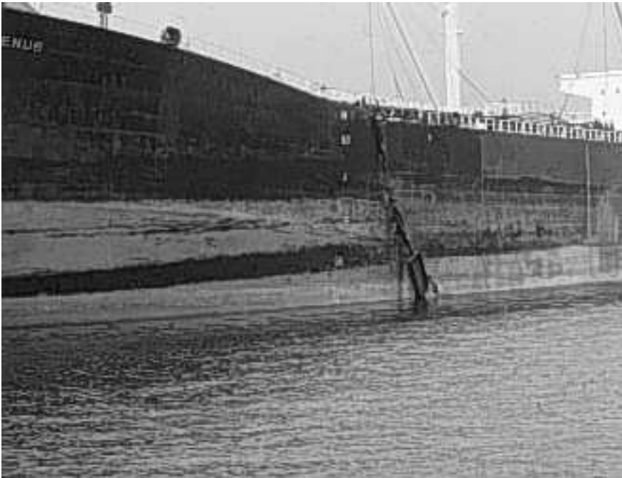
Figure 3.3: Alvenus buckled after grounding. Source: R. Hamm.
