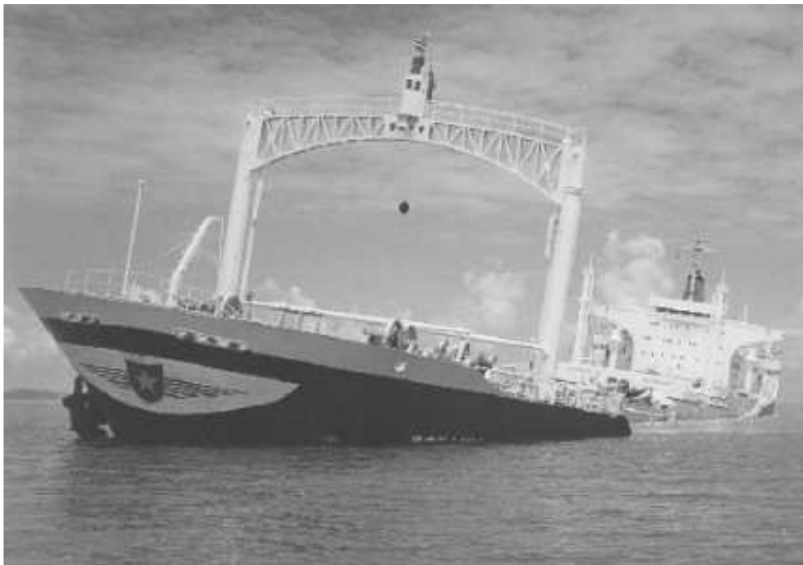
Figure C.6: Oceanic Grandeur after flooding. Hull is under extreme sagging moment but survived. No new tanker would. Note the extremely strong kingposts and the rare forward crowsnest, signs of an unusually well-sped ship. Source: Australian Maritime Safety Authority.
