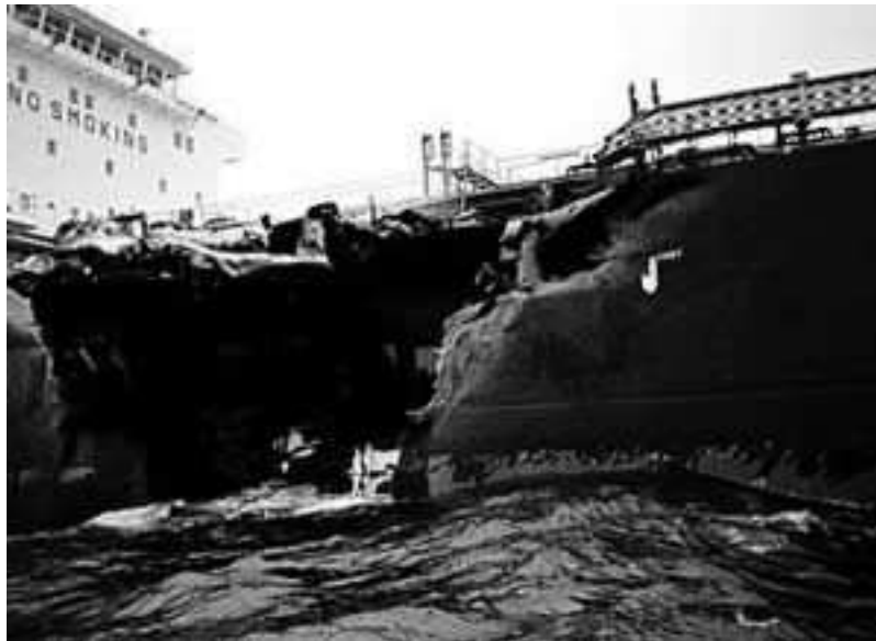
Figure 3.6: Close up view of Baltic Carrier penetration. Source: DR.
