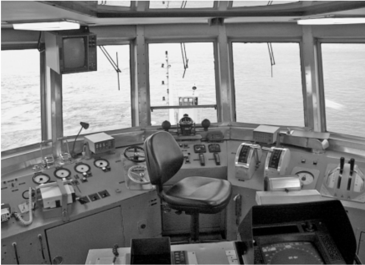
Figure 7. Pilothouse controls on ferry's Staten Island end. Thrust levers are on right of operator's chair, handwheels on left. Behind operator's chair (outside his field of view) is monitor for 10-centimeter radar display with automatic plotting aid showing other vessels' course, speed, and closest-point-of-approach. Data (blips) on 3-centimeter radar display (smaller screen behind operator) are repeated on monitor hanging above controls.
