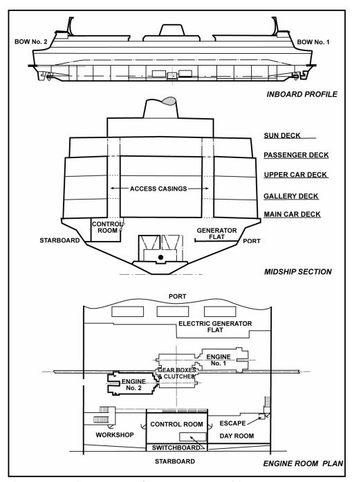
Figure 1. General arrangement of compartments at midships
