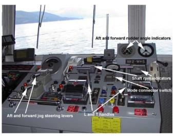
Photo 2. Wheelhouse control console
