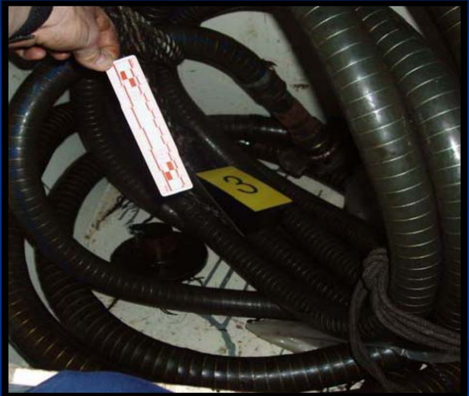
Portable Welden Pump and Flexible Rubber Hose Used to Bypass the Oil Water Separator
