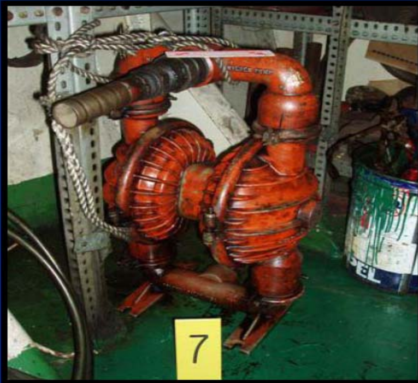
Portable Welden Pump and Flexible Rubber Hose Used to Bypass the Oil Water Separator
