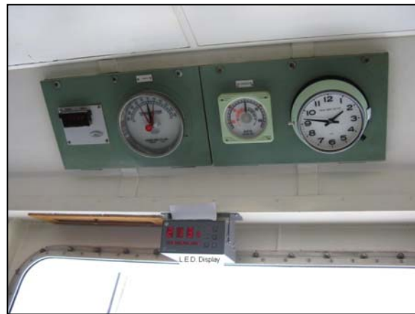
Photo 4. LED analogue repeater and rudder angle indicator.
