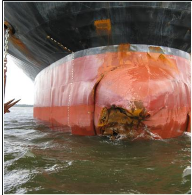
Photo 5. Damage to the bulbous bow.
