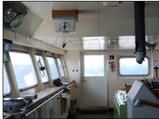
Photo 2. View of deckhead-mounted rudder angle indicator and magnetic compass reflector tube.
