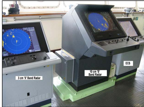
Photo 3. 3 cm radar, 10 cm radar and ECS.
