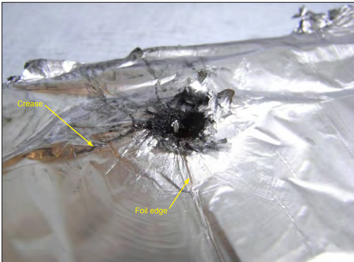
Crease on capacitor element
