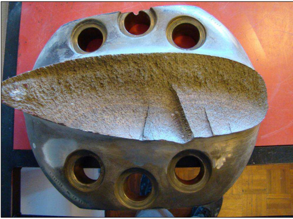
Figure 46: Fractured surface from the aft stern thruster blade base that was replaced by a new one in October 2012
