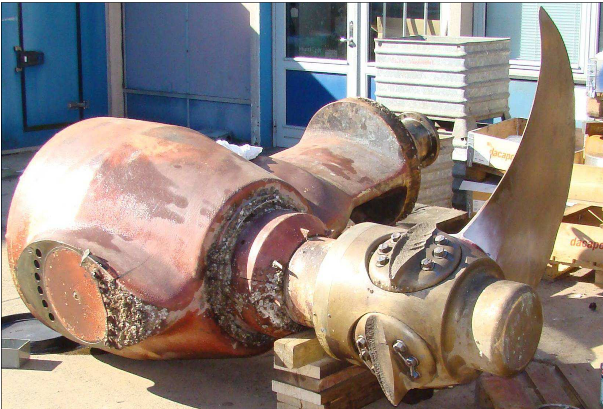
Figure 45: The damaged forward stern thruster before dismantling Source: FORCE Technology
