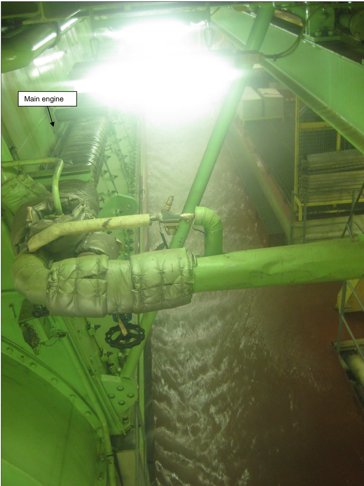
Figure 21: Engine room getting flooded Source: Maersk Line
