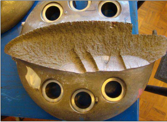
Figure 44: Fractured surface from the forward stern thruster blade base no. 4 Source: FORCE Technology
