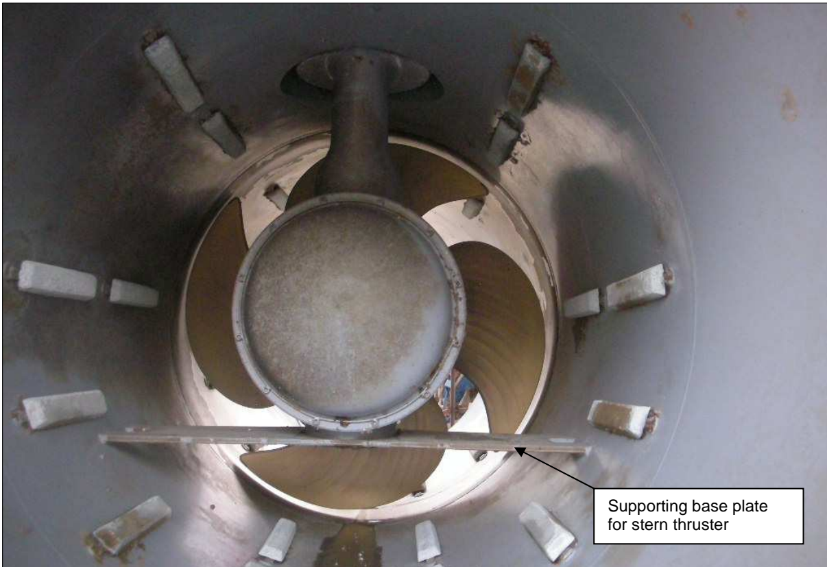
Figure 37: Stern thruster on a sister ship, viewed from the gearbox side Source: Maersk Line
