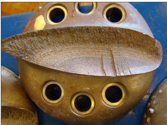
Figures 42 and 43: Fractured surfaces from the forward stern thruster’s blade bases no. 2 and no. 3 Source: FORCE Technology
