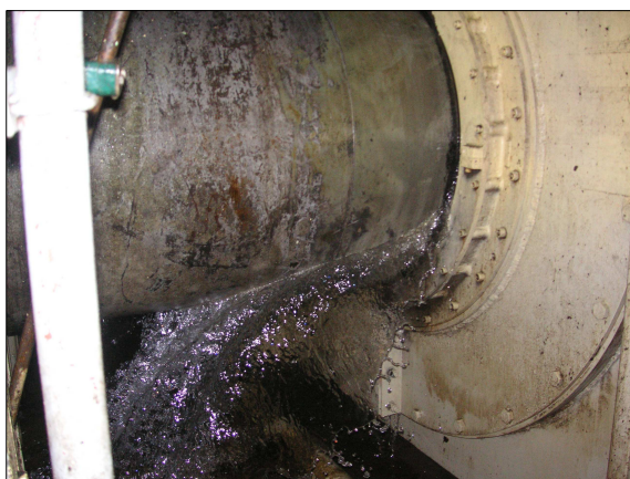
Figures 13 and 14: Ingress of water from the shaft tunnel to the engine room at the propeller shaft sealing when, at the repair yard, water in the engine room is being discharged and the propeller shaft tunnel is still flooded.
