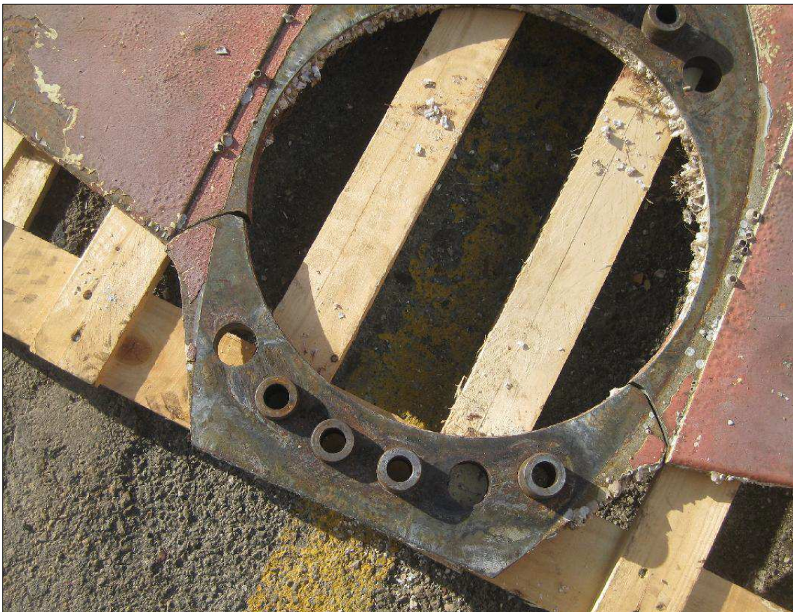
Figure 54: Fracture of supporting base plate for the aft stern thruster Source: BANDAK Engineering/Rolls Royce Marine
