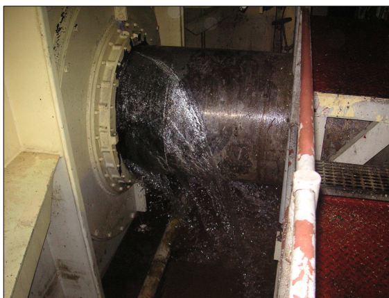
Figures 13 and 14: Ingress of water from the shaft tunnel to the engine room at the propeller shaft sealing when, at the repair yard, water in the engine room is being discharged and the propeller shaft tunnel is still flooded.
