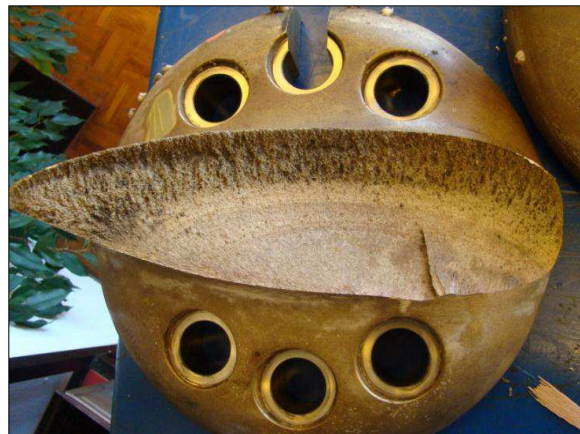
Figures 42 and 43: Fractured surfaces from the forward stern thruster’s blade bases no. 2 and no. 3 Source: FORCE Technology
