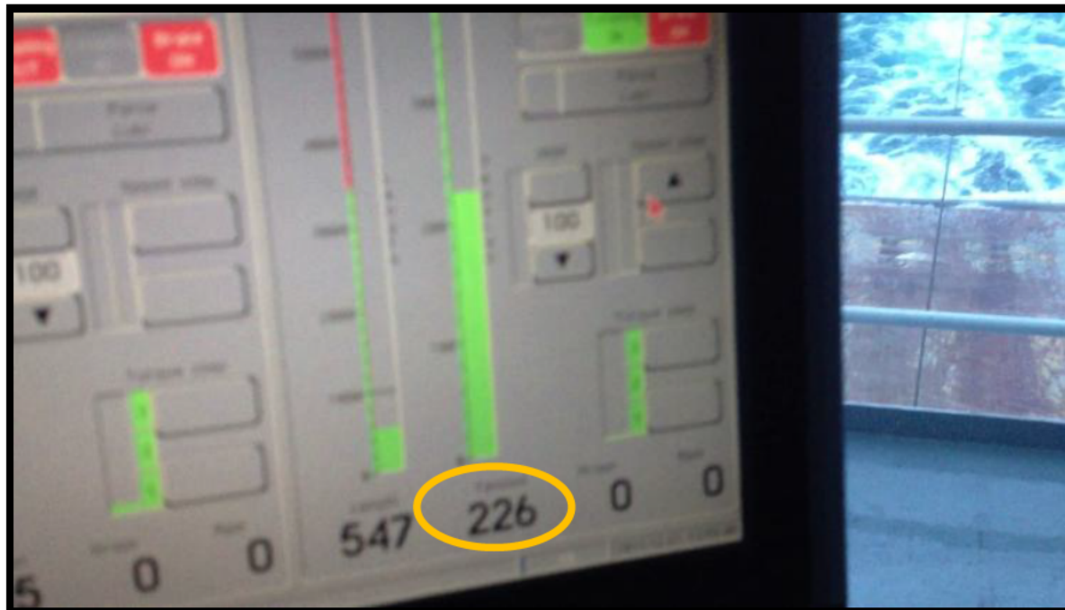
Figure 19: Screen capture from video showing tension reading of 226 tons on main tow drum. (Cell phone video screen capture provided by Mr. [REDACTED] AIVIQ Mate)
