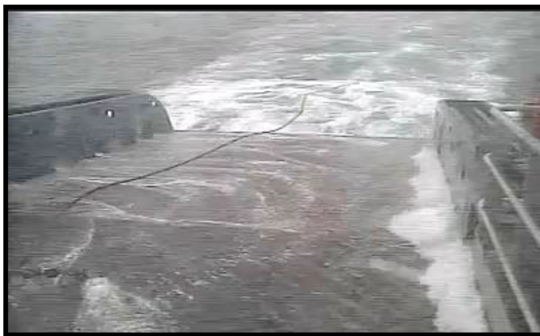
Figure 21: Screen capture of towline at moment of shackle failure on the morning of December 27, 2012 (From AIVIQ CCTV recording and provided by ECO)
