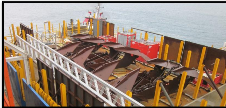
Figure 7: Five anchors stored aboard the KULLUK before transit. These were for use when the towing operation reached the Seattle Area while the KULLUK awaited dock space availability. (USCG Photo)
