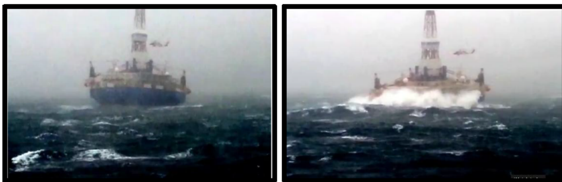
Figure 48: Screen captures showing extreme pitching resulting in the KULLUK burying hull into seaway and causing increased towing resistance. ( Taken from YouTube video taken by unknown AIVIQ crewmember during afternoon hours of 31 December with AIVIQ and ALERT towing, video titled “KULLUK rescue 2012 Gulf of Alaska” )
