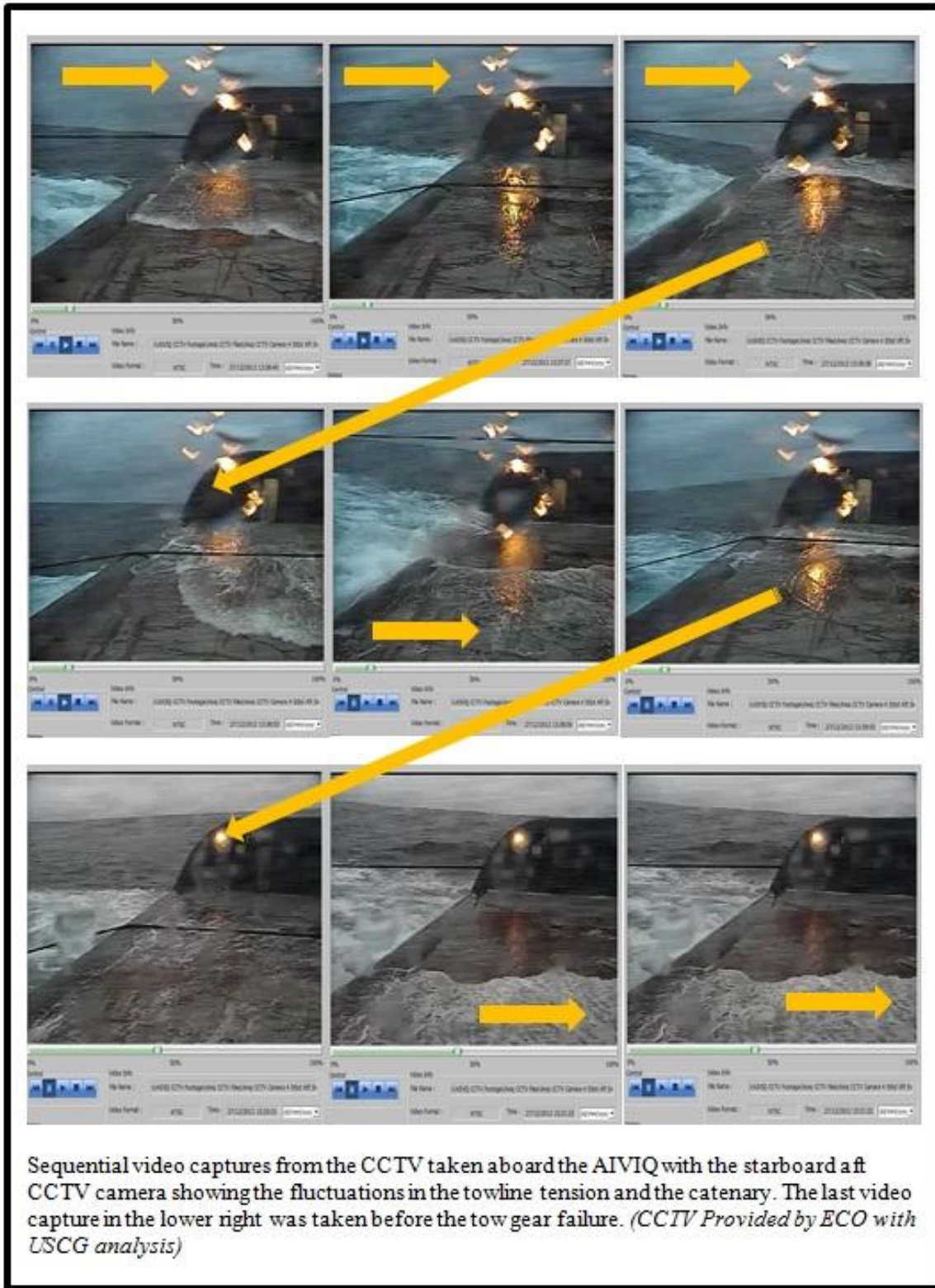
Figure 67 – Movement of AIVIQ towline and tension on the line on the morning of December 27, 2012.
