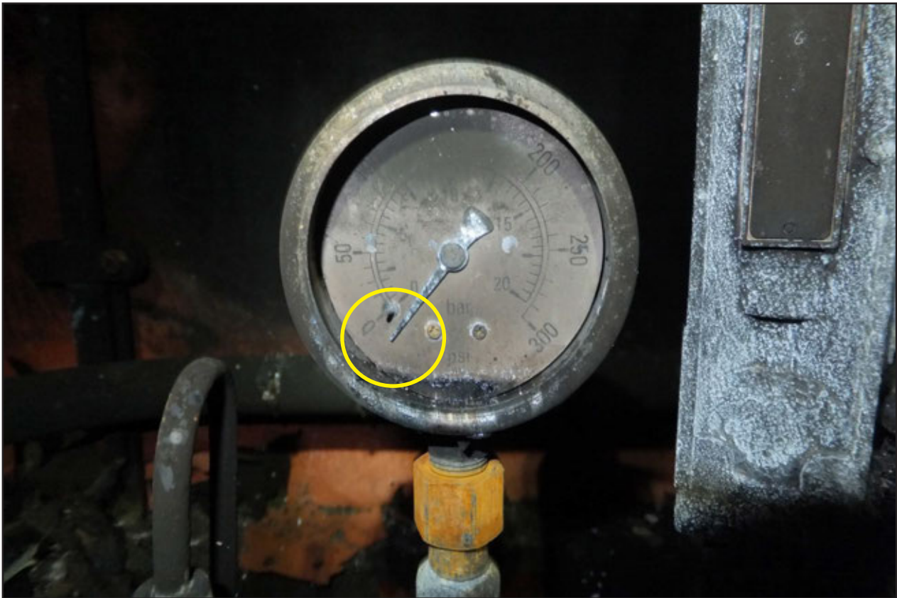
Figure 3: Starboard controllable pitch propeller system oil distribution box return line oil pressure gauge (PG3) (post-fire)
