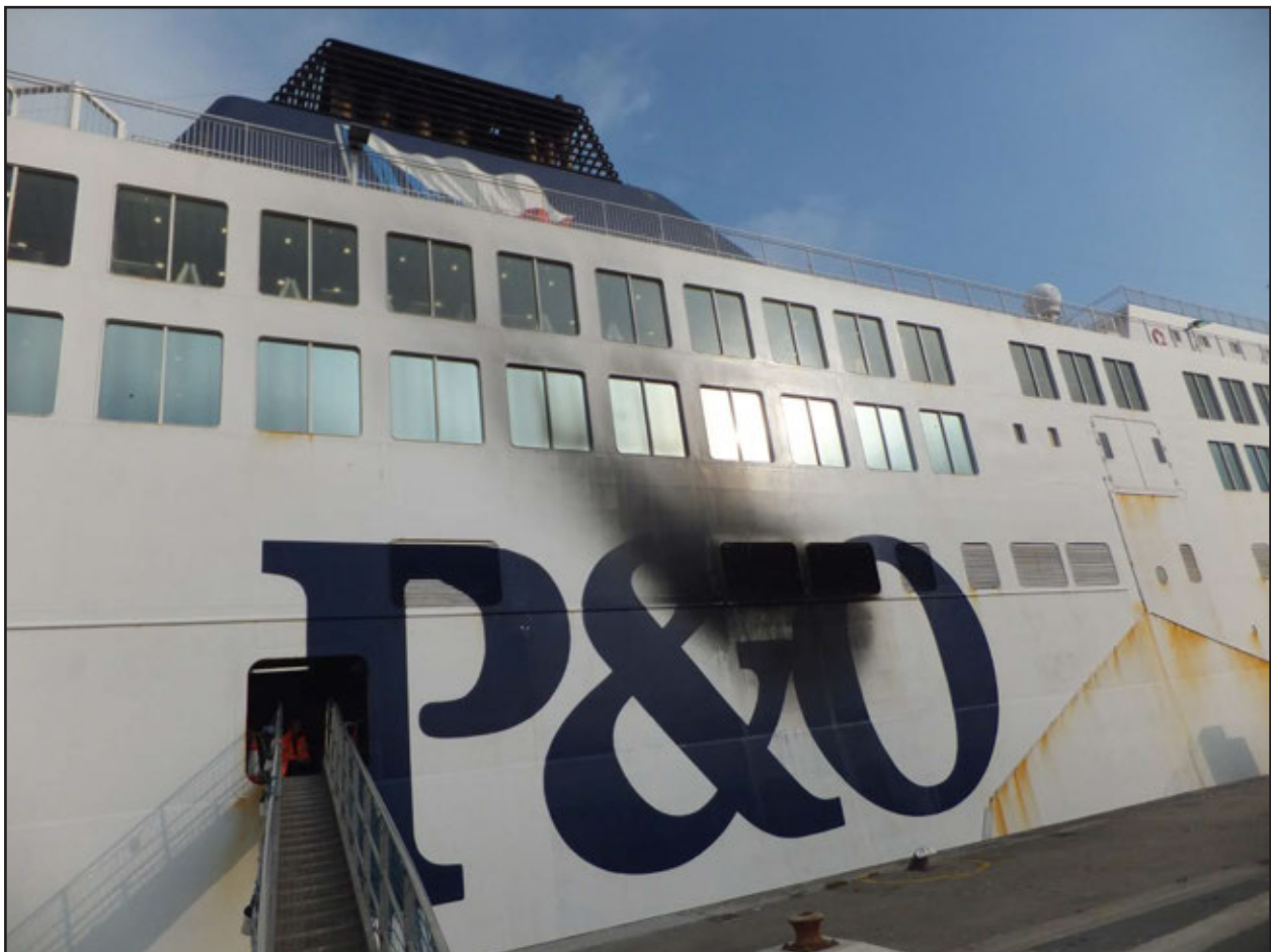
Figure 9: Smoke staining on starboard side
