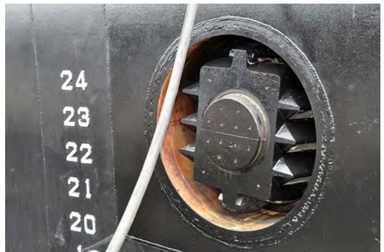
Figure 1: This is what the pins look like. One set is located on each side of the tug's bow.
