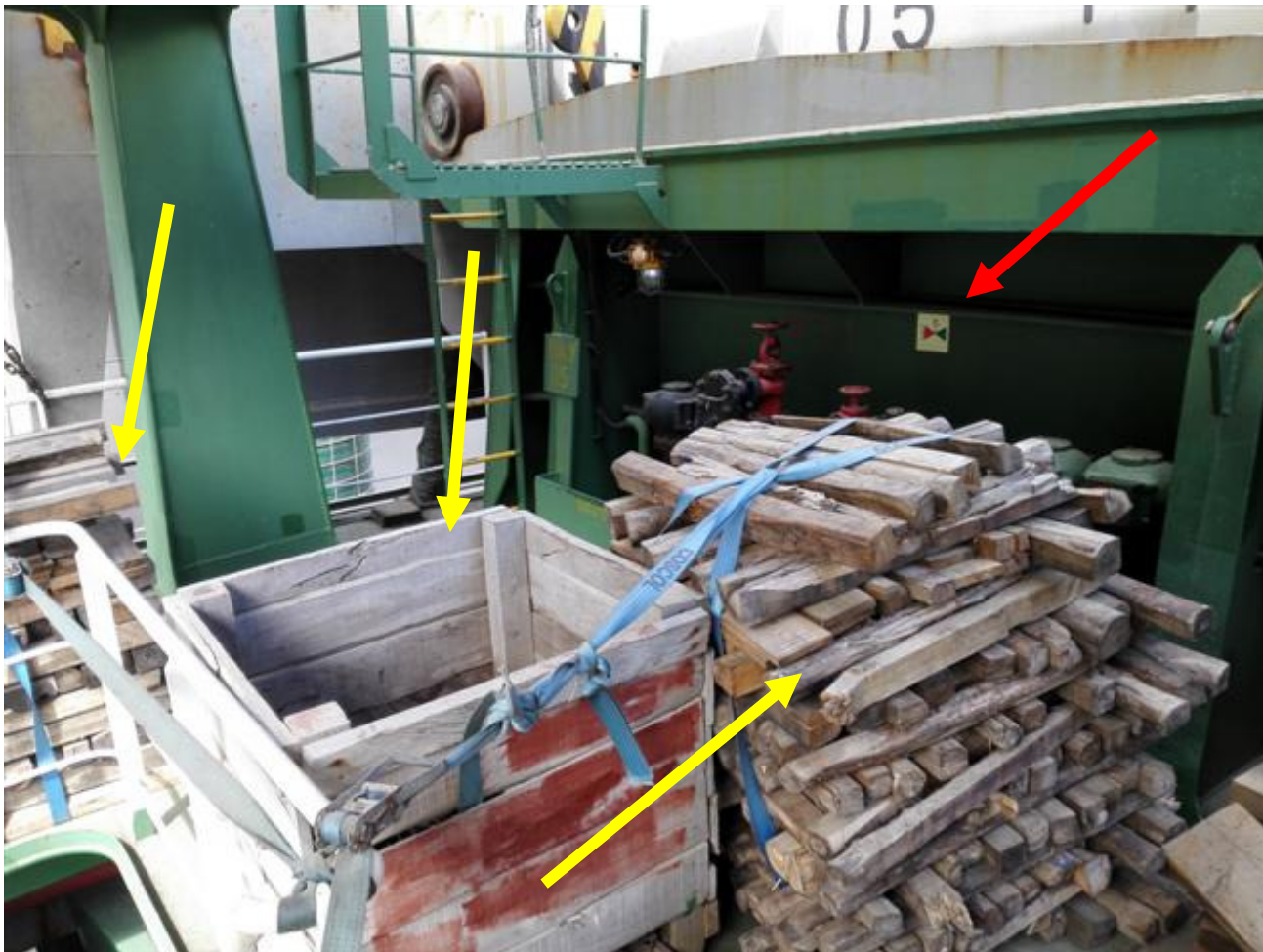
In this picture the fire fighting equipment is totally blocked by dunnage. Hydrants and also fire hose cabinets were not readily accessible at all. This deficiency was recorded with ground for detention.
