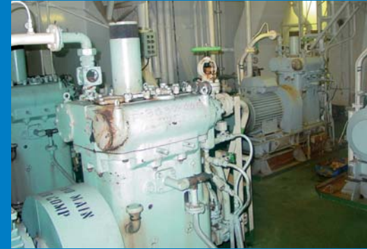
▶ Typical air compressors on a vessel
