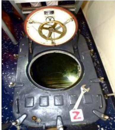
Figure 17—Scuttle and hatch into Berthing 4 showing the space completely flooded
