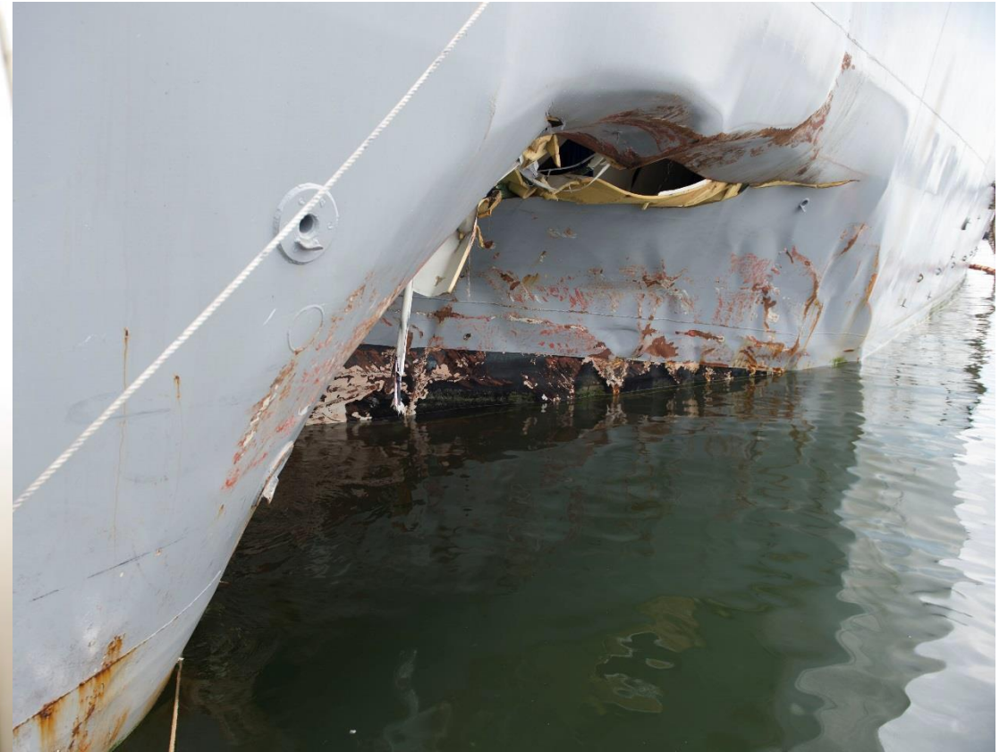
External view of point of impact; rupture in hull of the ship visible
