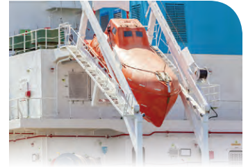
Exemplar enclosed freefall lifeboat in launch position on a slipway
