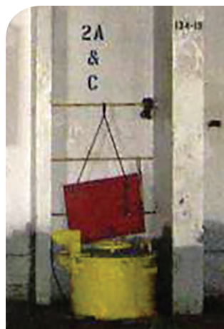
Second deck scuttle to hold 2A, similar to hold 3 scuttle Photo: Herbert Engineering
