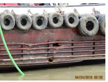
**Figure 68.** Punctures to the vessel's hull are visible. Source: Central Maritime, L.L.C.
