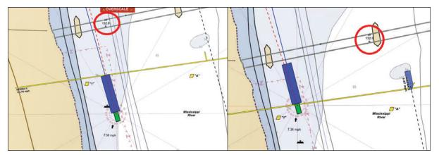
**Figure 88.** Screenshots of the *Kristin Alexis'* Rose Point at 0139 (left) and at 0140 (right). The vertical clearance for the Sunshine Bridge is circled in red.
