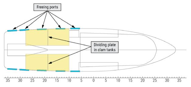
**Figure 9.** Plan view of *Misty Blue*'s tank layout and freeing port locations. The clam tanks are highlighted in yellow. Source: Coast Guard: Annotated By NTSB.
