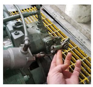
**Figure 101.** Starboard engine pneumatic gear clutch actuator linkage disconnected aboard the *Lindberg Crosby* as found after the accident.
