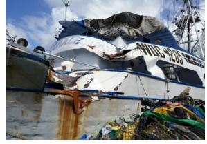
**Figure 11.** Damage sustained to both vessels. Bow of *American Eagle* (left) and *Koorale* (right). Source: American Eagle FISHING, LLC.
