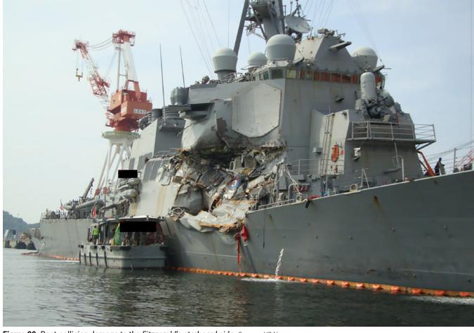
Figure 29. Post-collision damage to the Fitzgerald's starboard side. Source: US NAVY.
