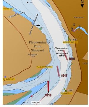
**Figure 100.** Screen capture from playback of *Leviticus'* navigation system at 1016 shows tow length and predicted positions as the vessel rounds the bend. Position times have been superimposed.
