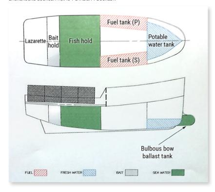
The probable cause of the sinking of the fishing vessel *Pacific 1* was the captain's decision to remain at sea with continuous flooding in the lazarette from an undetermined source, which accelerated and eventually led to progressive flooding.
