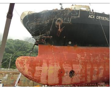
**Figure 33.** Postaccident damage to the *ACX Crystal's* bow. SOURCE: JAPAN TRANSPORT SAFETY BOARD.
