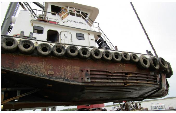
Figure 67. De Jeanne Maria during recovery. Punctures to the vessel's hull are visible. Source: CENTRAL MARITIME, L.L.C.
