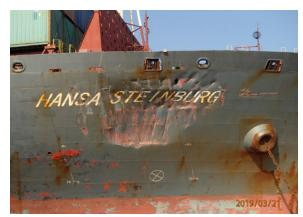
**Figure 18.** Damage to *Hansa Steinburg* starboard-side bow. Source: Coast Guard.
