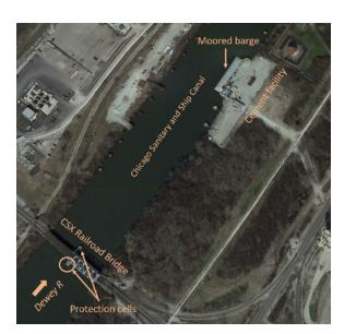
**Figure 70.** Location of the Chicago Sanitary and Ship Canal where the *Dewey R* and tow attempted to pass through the CSX Railroad Bridge, and location of a barge moored at the cement facility, similar to the barge that was moored at the time of the accident. The protection cell that was struck is circled. Background source: Google Maps.
