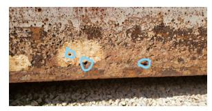
**Figure 159.** An annotated photo from the vessel company identifies holes on the side shell of the barge near the bottom plating. Source: HEX STONE.
