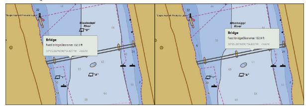
**Figure 89.** Vertical clearance of the Sunshine Bridge's west (left) and channel (right) spans, as indicated postaccident by the Rose Point display on board the *Kristin Alexis*, which showed the same clearance for each span (132.9 feet).
