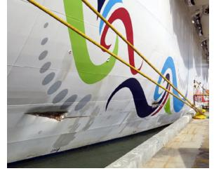
Figure 112. Damage to the Norwegian Epic's hull.
