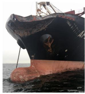
Figure 15. Damage to APL Guam. Source: Coast Guard.
