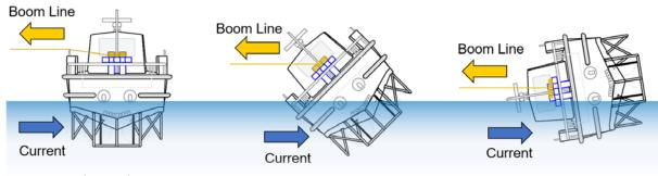
**Figure 6.** The forces of the current and boom towline acting to capsize the MSRC 8-1.
