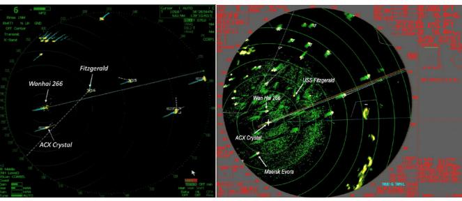
**Figure 32.** A comparison of radar screens from different vessels before the collision. **Left:** Screen capture from the *Wan Hai 266* electronic navigation software, about 6 minutes before the collision. **Right:** Screen capture from the *ACX Crystal* electronic navigation software (radar and ARPA), at the same time. (Vessel names have been added to screen images.)
