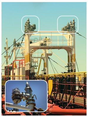
**Figure 183.** PV valves on board the main deck of the *Fairchem Filly*.
