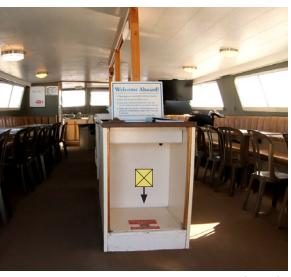
**Figure 139.** The bunkroom escape hatch, viewed from aft in the salon on the main deck.
