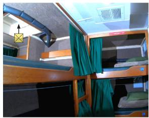
**Figure 140.** The escape hatch, viewed from the bunkroom below deck. Source: R. CLEVENGER, ANNOTATED BY NTSB.
