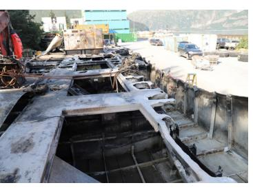
**Figure 127.** Bent and deformed deck plating forward on the *Alaganik*'s starboard pontoon after the fire.
