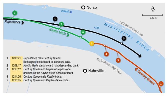
**Figure 23.** Tracklines of the vessels during the last 7 minutes prior to the collision. The *Century Queen* is represented in red, the *Kaytlin Marie* in green, and the *Repentance* in black. Background source: Google Maps.
