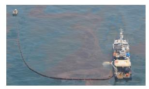
**Figure 4.** J-configuration deployment of oil spill boom by MSRC OSRV (right) and 32-foot workboat (left) during *Deepwater Horizon* oil spill response in May 2010.
