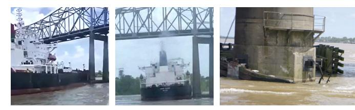
**Figure 65. Left and middle:** Two photos showing the *Dank Silver* striking the Sunshine Bridge. Source: Crescent Towing. **Right:** Damage to the fendering system for the western pier of the Sunshine Bridge, from the north.
