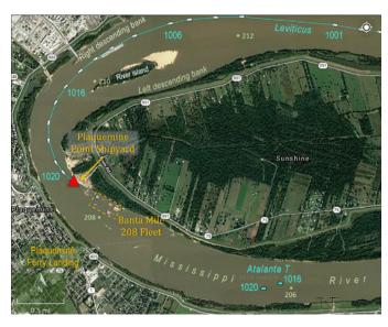
**Figure 96.** Trackline of *Leviticus* leading up to the contact with the barges moored at the Plaquemine Point Shipyard, based on the vessel's AIS data. According to the passing arrangement, Plaquemine Ferry Landing is where the tow would have met the *Atalanta T*.
