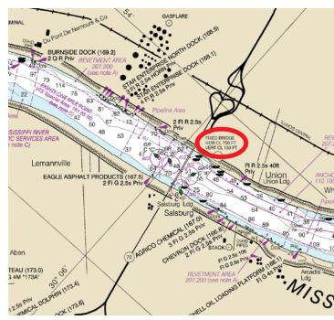
**Figure 93.** Excerpt of NOAA chart 11370 used by the crew. The vertical (133 feet) and horizontal clearances (750 feet) of the Sunshine Bridge are shown circled in red. SOURCE: NOAA: ANNOTATED BY NTSB.
