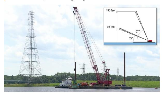
**Figure 86.** Towing vessel *Goose Creek* and crane barge *U1510* spudded down in Chesapeake, Virginia, after the accident. Inset (not to scale) depicts the crane boom elevation when stowed at 22° and as determined after the accident with an angle of 67°. Source: Coast Guard; ILLUSTRATION BY NTSB.
