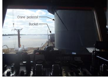
**Figure 92.** Forward view from the *Kristin Alexis'* wheelhouse. The crane's pedestal blocks most of the starboard view, while the crane bucket blocks a portion of the forward view ahead.
