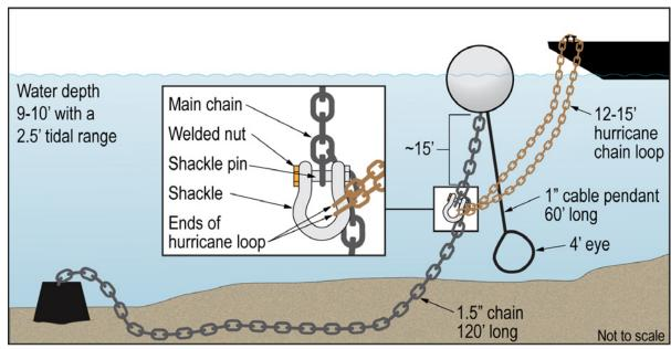
**Figure 126.** A representation of the arrangement of the *YD 71*'s mooring at the time of the accident.
