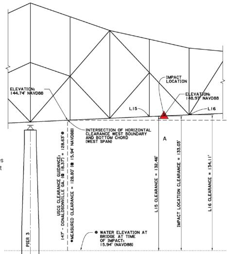
Figure 95. Vertical clearances of the Sunshine Bridge's west span measured shortly after the accident. The impact location is marked with a red triangle.
