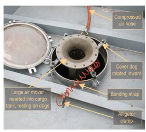
**Figure 151.** Demonstration of air-mover-installation methods reconstructed after the accident. **Left:** Smaller (6-inch diameter) air mover without compressed air hose and bonding wire. **Right:** Larger (11-inch-diameter) air mover connected with compressed air hose and bonding wire with clamp.
