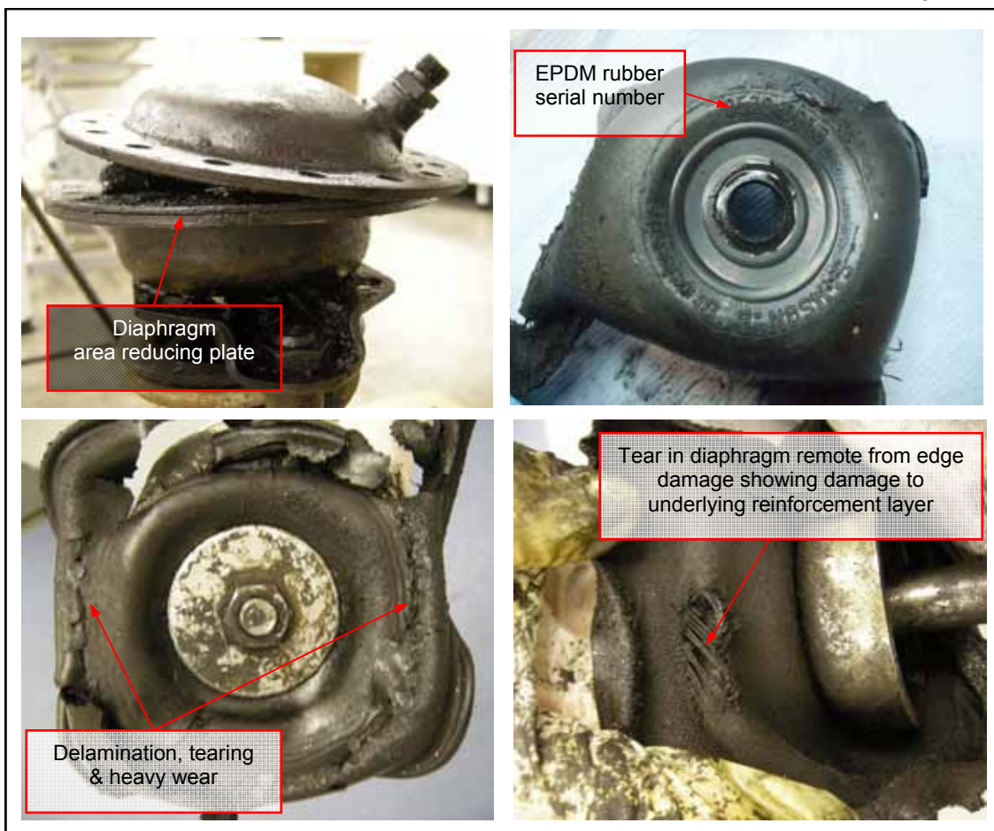
Condition of the auxiliary engines' excess fuel pressure regulating valve diaphragm
