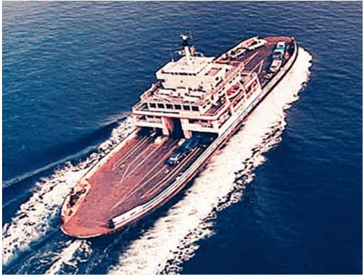
**Figure 1.** Aerial view of vessel showing wheelhouse, vehicle deck and double ended features.
