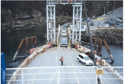
**Figure 3.** View of vehicle deck and a loading operation as the ferry is pushing against the wing walls of the dock.
