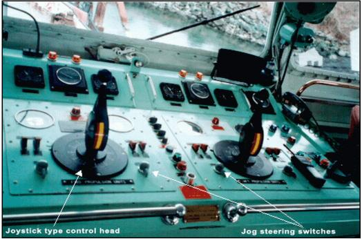
**Figure 4.** View of control console showing control heads, jog steering and rudder angle indicators.
