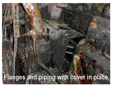
32" after recognizing that "during the long life span of VASA 32 engines some incidents of serious fuel leakage in the low pressure fuel supply have occurred and a few of the leakages have led to a fire." The bulletin recommended modifications to different components of the fuel oil systems on the engine. Information was provided on new types
