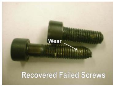
residual load to maintain the seal. The fuel line flange was designed for screws 30 mm long yet after the casualty a much longer screw requiring spacers was found. Additionally other improperly sized screws were observed on flanges of the number three main engine crossover piping.
