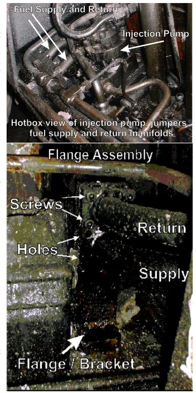
Only one screw remained which freely allowed movement of the pipe and facilitated separation at the flange. The sealing of the flange was accomplished by using an o-ring recessed in a groove machined into the surface of the piping flange.
