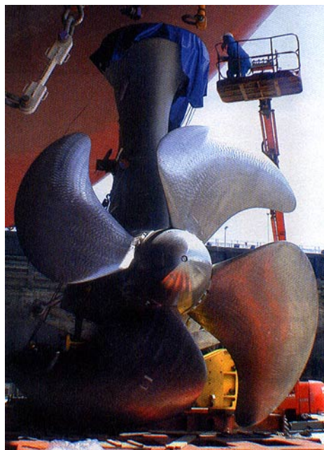
The mermaid pods were fitted in Basin C after the ship had been floated out of the building dock.
