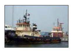
Files TG20137 / TG20140 Twin Screw Tugs (2) 29.0m / 26.5m x 9.0m x 4.25m depth / 3.9m max draft. Built 1999 by Jiangdu Yuehai Ship; China. Singapore flag. G/NRT 247/74. ABS +A1 (E) Towing, +AMS thru Oct '09 / Jul '09 resp.
