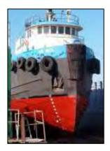
Marcon International's first sale of '08 was the 2,000BHP twin screw "Mr. Nick" bought by E.J. Ventures, LP of Texas from Moby Marine of Florida. Tug was built in 1976 by Slocum Iron Works, Mobile, Alabama and measures 99.5' x 31' x 17' depth with an ABS Loadline
