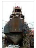
house, stern section and propulsion system. Her existing EMD 12-645C 1,500HP engine, Falk gear and single 104" 4-blade stainless steel prop was replaced with two 228 General Electric 8 cylinder
