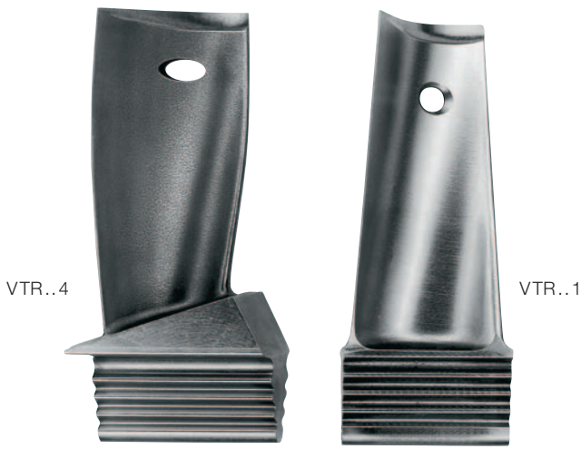
Fig. 9: Turbine blades with profile twisted from root to tip to take account of the increase in blade speed with the blade length.
