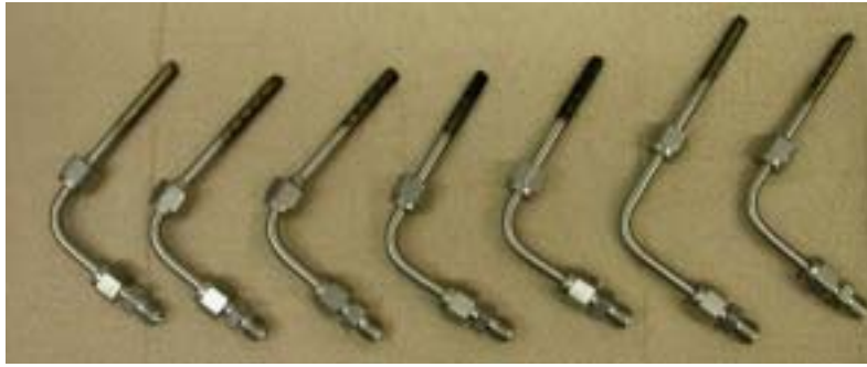
Figure 55: EGR Sampling Probes after 50 Hours of Operation
