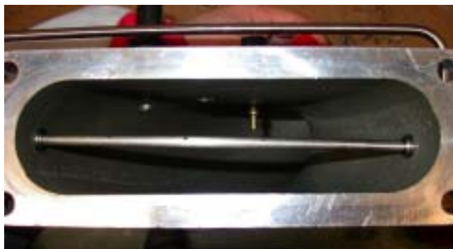
Figure 52: EGR Probe #1 in Intake Air Horn
