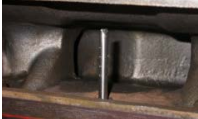
Figure 53: Typical “Pepper Pot” Sample Probe Installed in Cylinder Head
