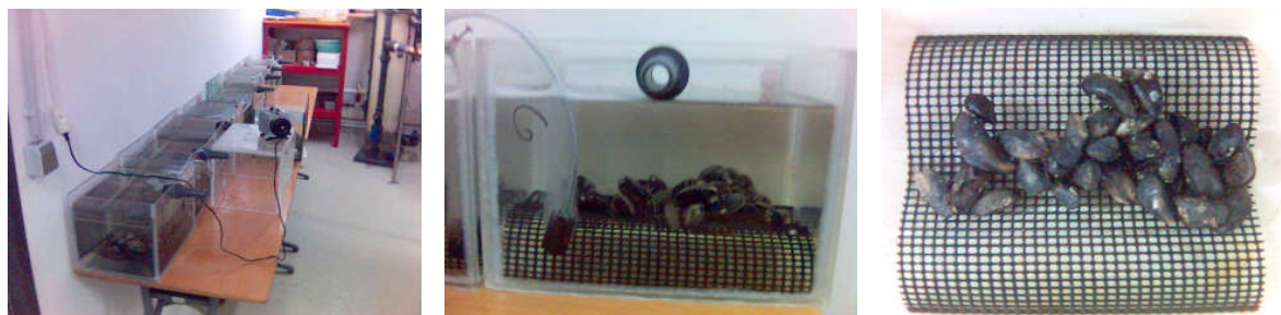
Fig. 7: Photographs of the experimental design of the accumulation test. L.: all nine aquariums with aeration pump. M.: close view on to an aquarium with aeration stone and mussels placed on the PVC net. R.: mussels on PVC net.
