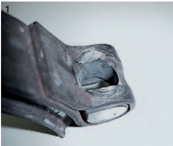
1 Severe wear at screw-head | 2 Deformed or wrong washer | 3 Cover tape detached | 4 Cover tape severely deformed
