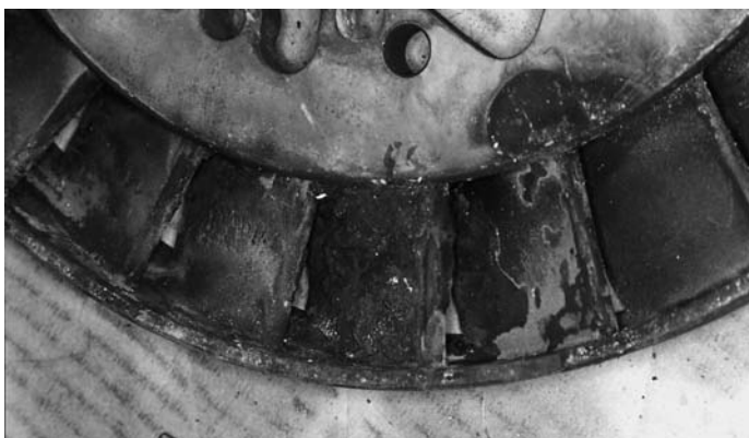
Dirty nozzle ring. Cleaning was not carried out according to our recommendations.
