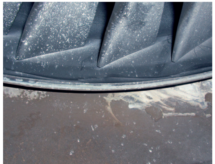
Worn turbine blade tips and turbine diffuser.
