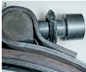
1 Severe wear at screw-head | 2 Deformed or wrong washer | 3 Cover tape detached | 4 Cover tape severely deformed
