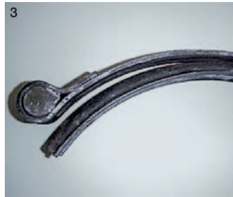
1 Severe wear at screw-head | 2 Deformed or wrong washer | 3 Cover tape detached | 4 Cover tape severely deformed
