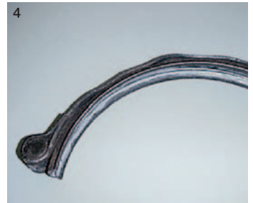
1 Severe wear at screw-head | 2 Deformed or wrong washer | 3 Cover tape detached | 4 Cover tape severely deformed
