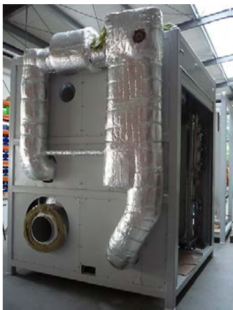
Figure A.3: The media module containing support systems for the fuel cell
