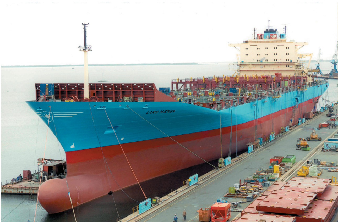
Fig. 1: The 3700 TEU container ship Lars Mærsk powered by a Sulzer 8RT-flex96C engine of 45,760 kW is seen here nearing completion at Odense Steel Shipyard A/S in Lindø, Denmark. [04#130]
