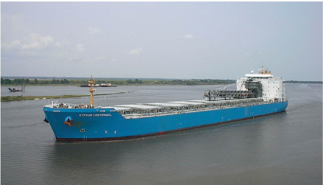
Fig. 9: The 47,950tdw self-unloading bulk carrier Gypsum Centennial of Gypsum Transportation Ltd powered by the first Sulzer RT-flex common-rail engine. [04#117]
