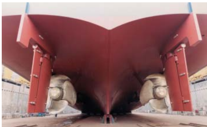
Fig. 1 Propulsion installation for a typical Ropax ferry.
