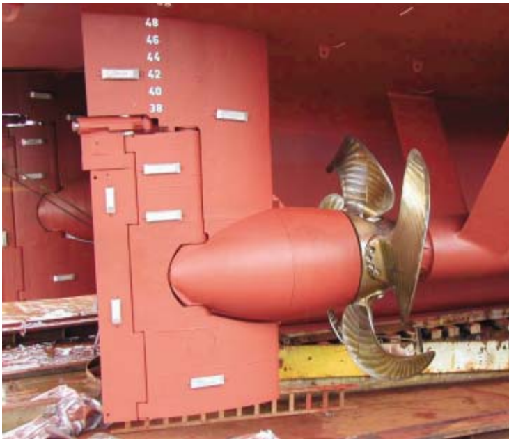
Fig. 9 The Efficiency Rudder on a twin-screw vessel.
