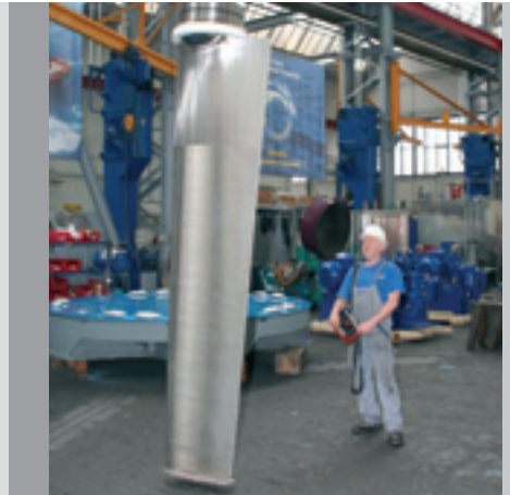
Fig. 15: The 3 m blade of a VSP for a PSV
