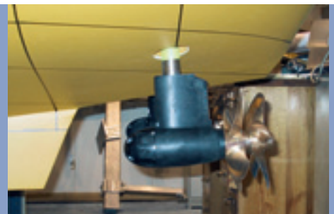
Fig. 8: Position of CRP in the stern of the PSV model
