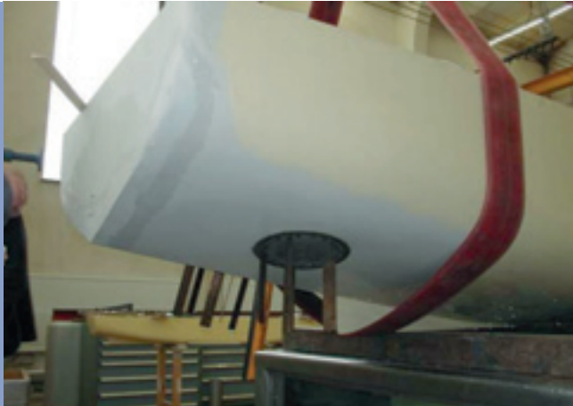
Fig. 10: Modified aft body with VSP installation
