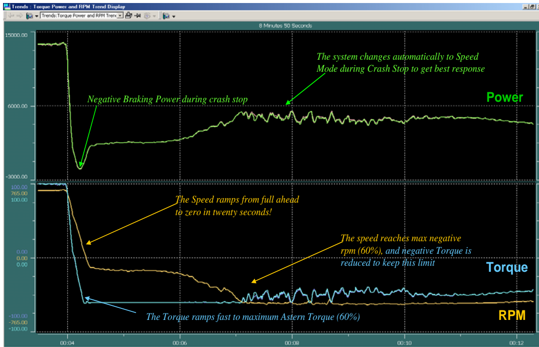
Figure 9. Propulsion motor power, RPM and torque at Crash Stop Test.
