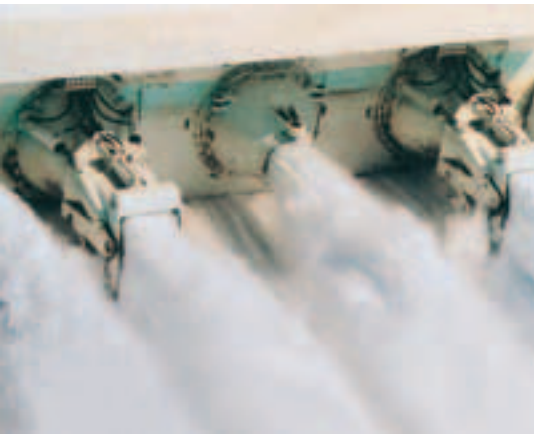
Figure 4: Waterjets in operation at the stern of a fast ferry
