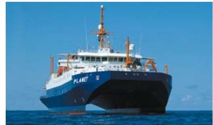
Research & trial vessel "Planet" with permanent excited propulsion motors 4 x 1040 kW and permanent excited main alternators
