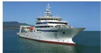
Research vessel "Sagar Nidhi" with PWM Active Front End (AFE) propulsion drives 2 x 1600 kW and 2 x 800 kW
