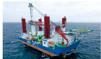
Jack-up vessel "Windlift I" with PWM Active Front End (AFE) propulsion drives 4 x 1100 kW
