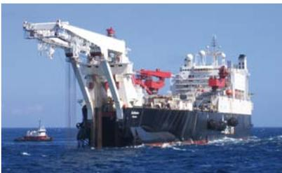
Pipe layer "Solitaire" with LCI propulsion drives 10 x 4.3 MW
