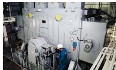
Propulsion motor 15 MW, 135 rpm on cruise liner "Norwegian Sun"
