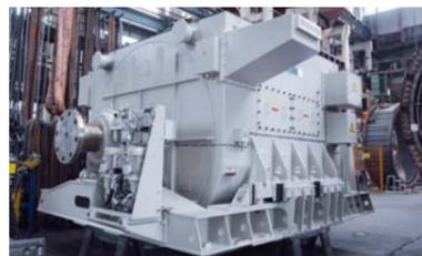
Propulsion motor 8.5 MW, 150 - 160 rpm on cruise liner "Silver Spirit"
