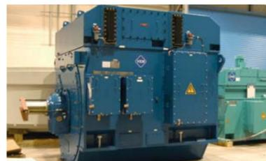
Main alternator 6920 kVA, 720 rpm on cruise liner "Seabourn Odyssey"
