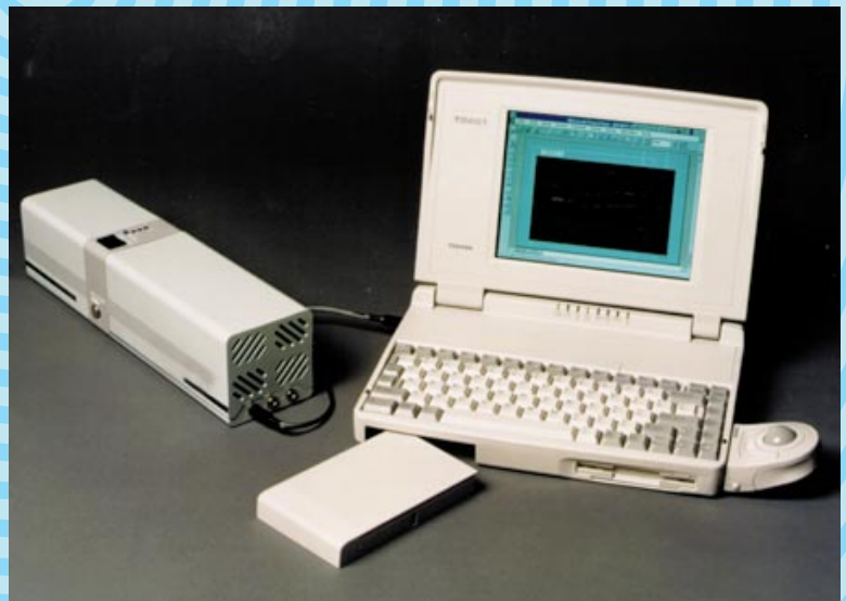
A laptop computer using a fuel cell power source can operate for up to 20 hours on a single charge of fuel. (Courtesy: Ballard Power Systems)
