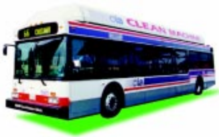
In March 1998, Chicago became the first city in the world to put pollution-free, hydrogen fuel cell powered buses in their public transit system. (Courtesy: Ballard Power Systems)
