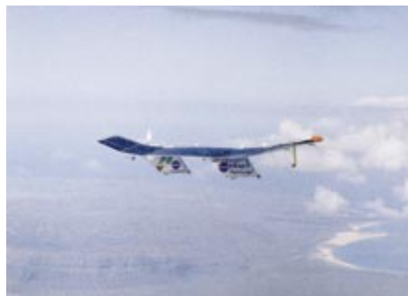
Unmanned solar plane powered by a renewable regenerative fuel cell (Courtesy: Aerovironment)
