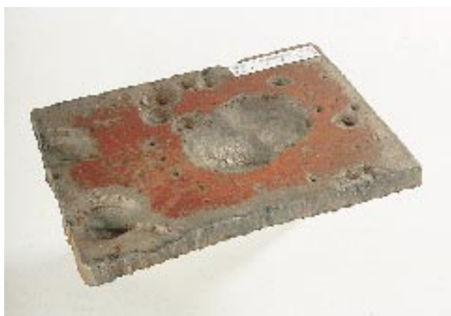
Figure 6.4 Ballast tank corrosion indicating extent of steel wastage after cleaning
