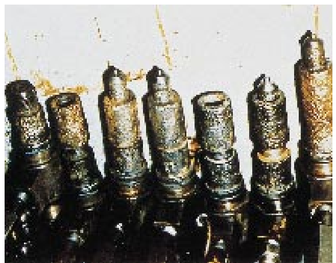
Figure 2.10 Sulphate reducing bacteria corrosion of fuel injectors
