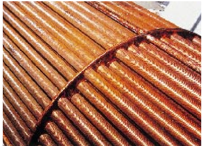
Figure 3.10 Lubricating oil cooler (oil side) corrosion of tubes and stays
