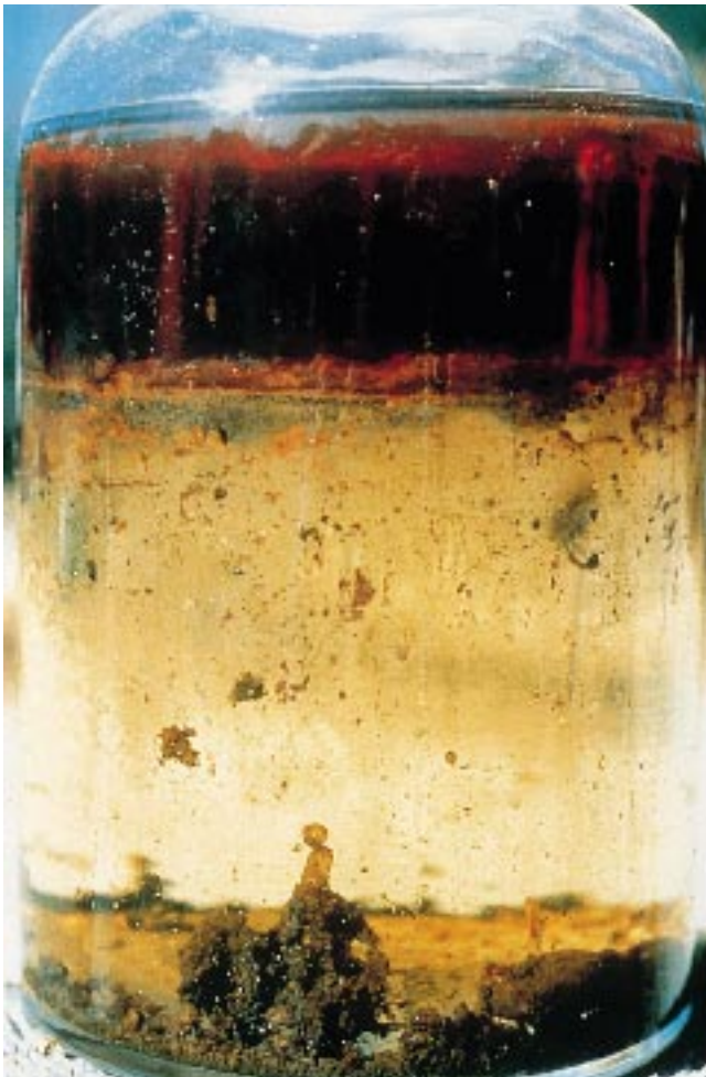
Figure 4.2 Contaminated fuel oil after being allowed to settle
