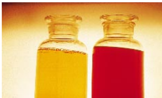
Figure 2.14 Contaminated fuel oil indicated by its haziness appearance
