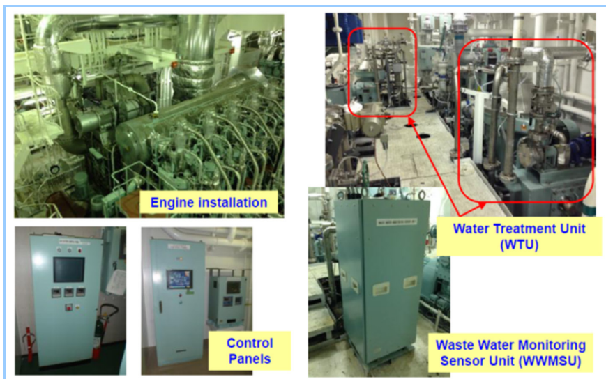
Figure 11 LP-EGR system installed into the actual ship
