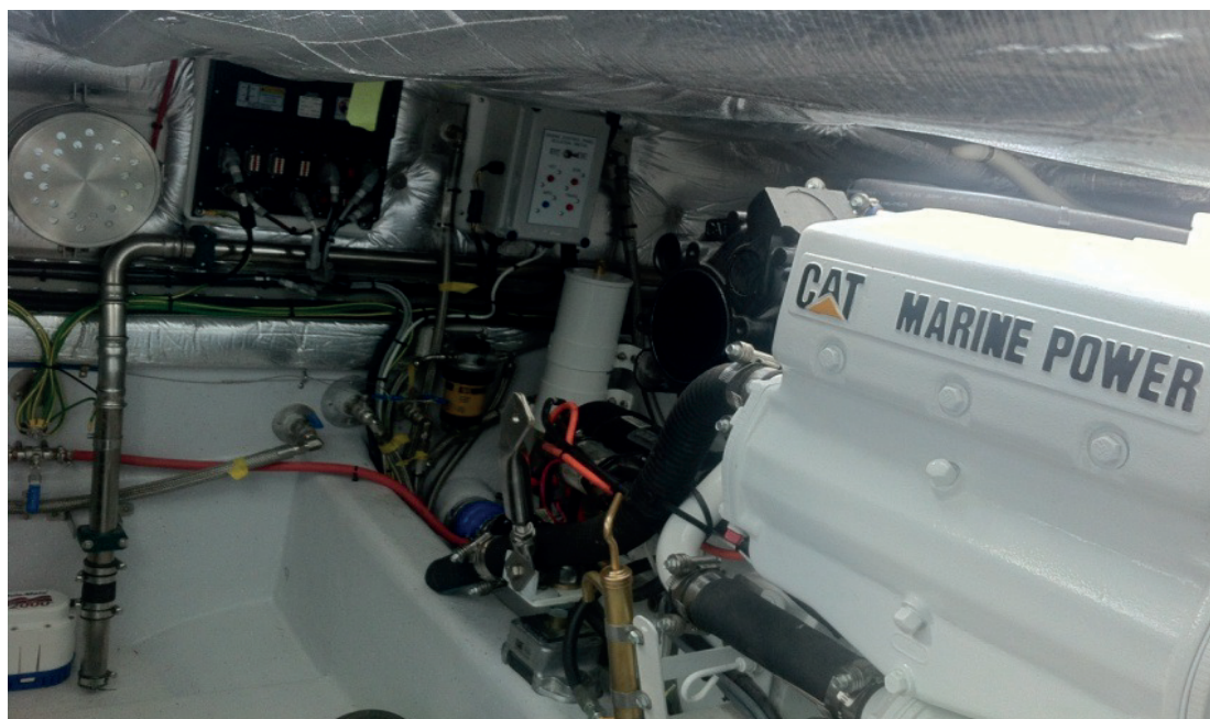
Figure 6 – Aerosol generator fitted in a small craft machinery space (top left of photograph)
