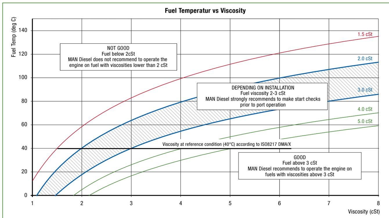
The horizontal axis shows the bunkered fuel viscosity in cSt, which should be informed in the bunker analysis report. If the temperature of the MGO is below the lower red curve at engine inlet, the viscosity is above 3 cSt.
