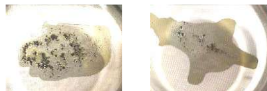
Fig 5. 60mesh filtration residue Left: MGO alone Right: ExtRS (10%)
