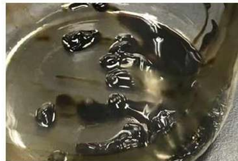
Wax collected in a metal scoop Source: Guide for use of 2020 SOx regulation compliant fuel oils (Maritime Bureau of the Ministry of Land, Infrastructure, Transport and Tourism of Japan)
