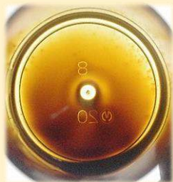
Image1 No sludge formation in compatibility of VLSFO (sludge does not occur)
