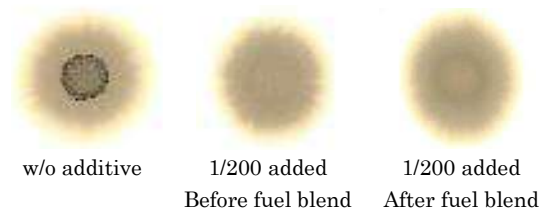
Figure 2. Influence of timing of SD-20 addition to mixed fuel (HSFO/LSMGO=1/8, w/w)
