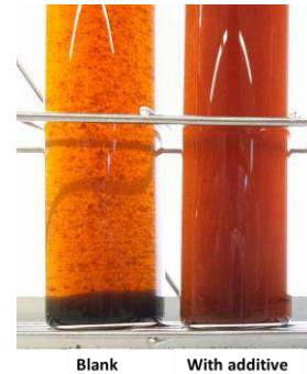
Fig. 3. Dispersion test with n-heptane.
